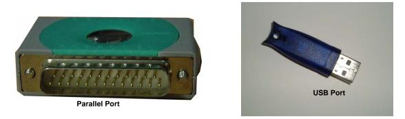
Figure 2-3: Liquid blue Dongles
